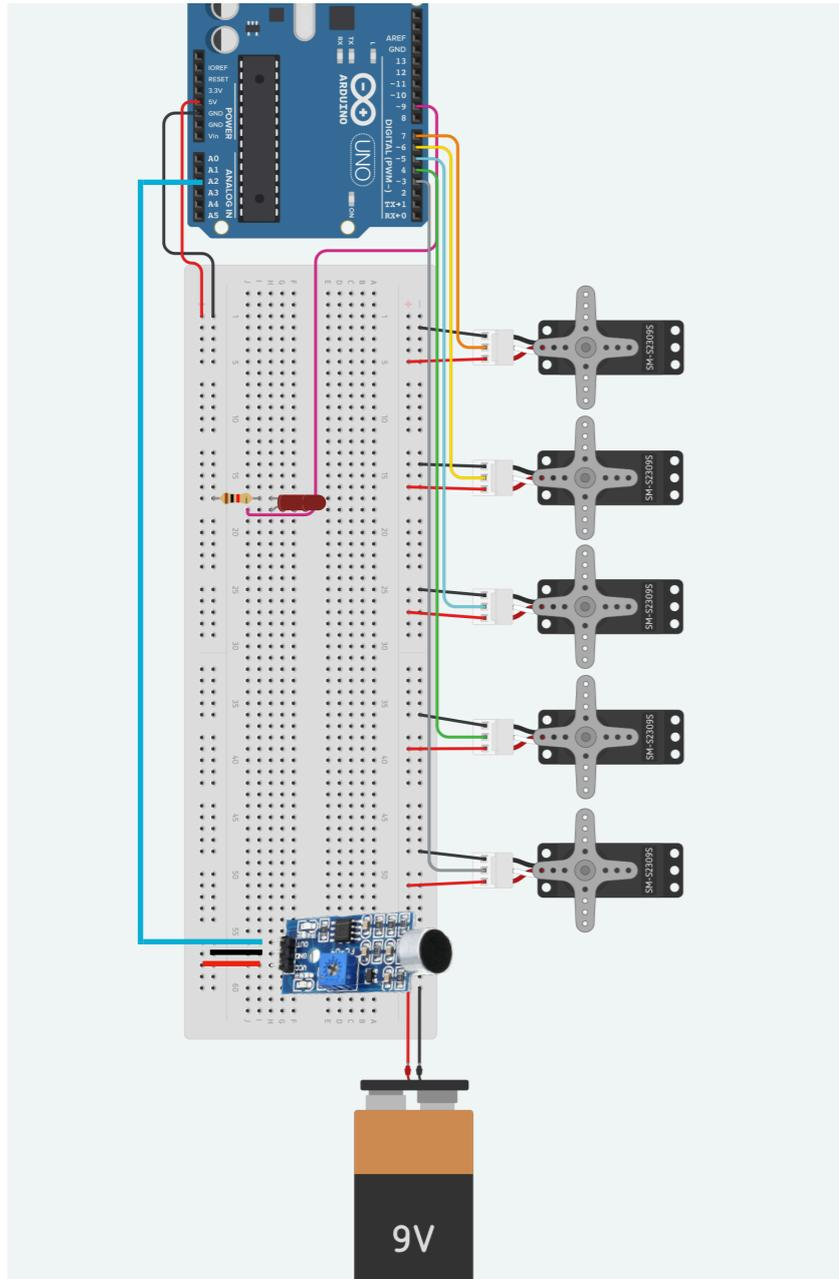
This is the TinkerCAD circuit for this project, with the 5 motors, the sound sensor, and the three LED lights.
